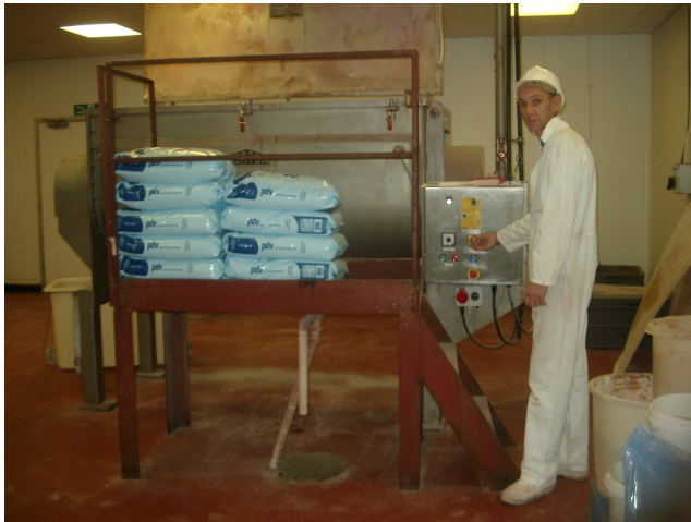
Above Raymond beside the Morton blender – a machine built in Newmains that is used to mix all McAusland Crawford recipes.
